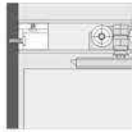
ZSL05 PVC Wall to Track Connector
